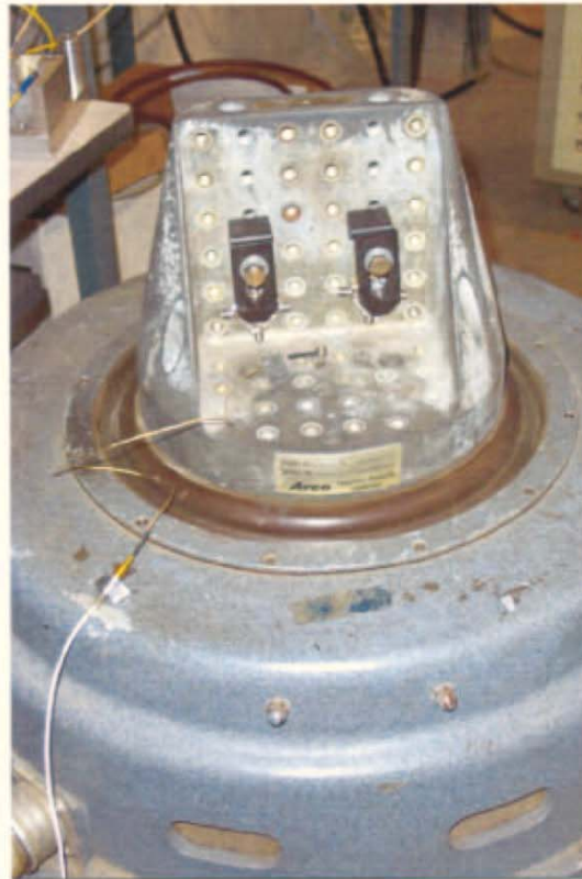
Photograph 3: View of Transverse Axis Vibration Test set-up
