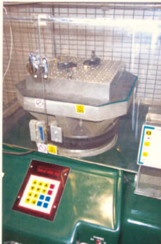
Photograph 4: View Positive Vertical Axis Shock Test set-up
