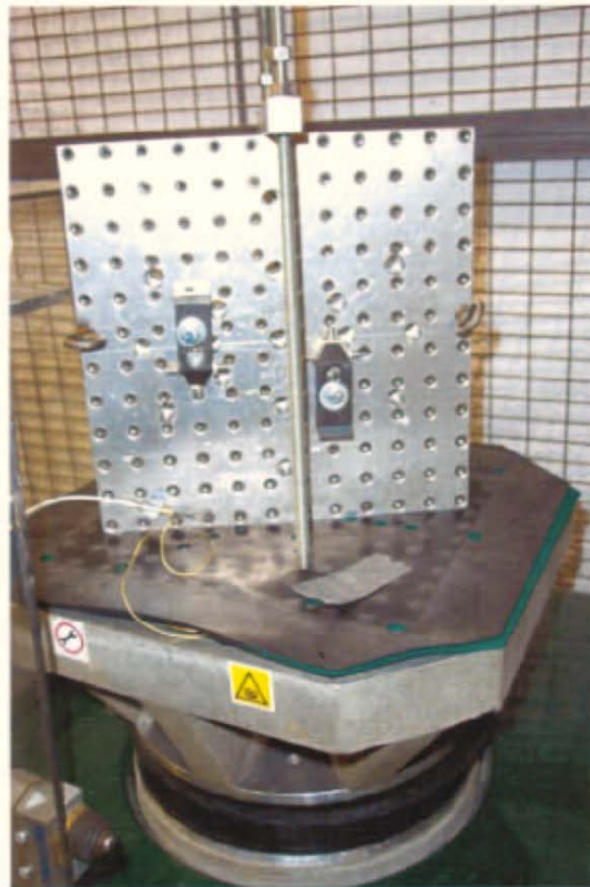
Photograph 9: View of Negative Transverse Axis Shock Test set-up
